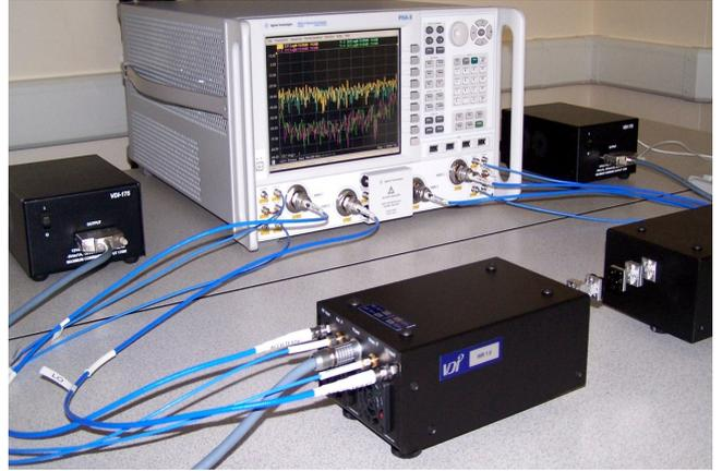
Figure 2: The 750 GHz to 1.1 THz VNA system used for the measurements
