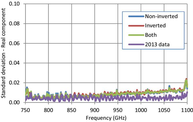
Figure 7:  $s(\Gamma_{R_i}^N)$ ,  $s(\Gamma_{R_i}^I)$  and  $s(\Gamma_{R_i}^{IN})$  for the near-matched load. Also shown are the results from 2013
