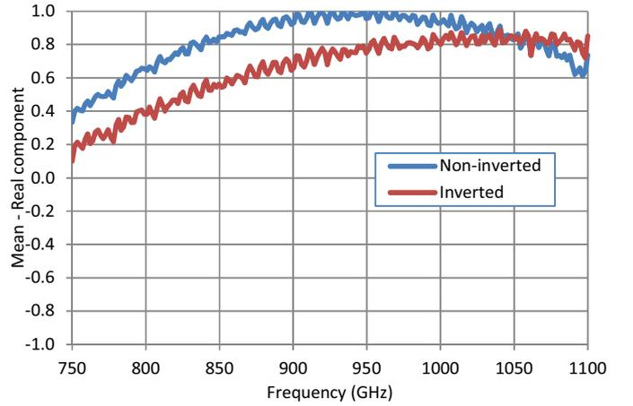
Figure 9:  $\bar{\Gamma}_R^N$  and  $\bar{\Gamma}_R^I$  for the offset short-circuit
