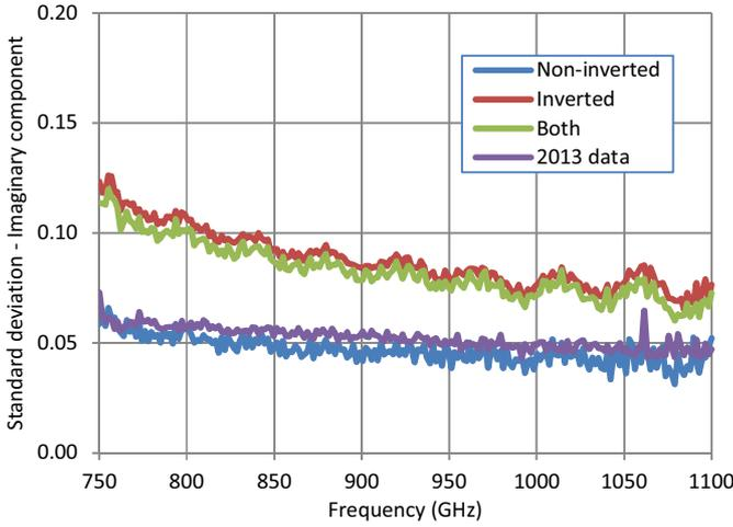
Figure 6:  $s(\Gamma_{I_i}^N)$ ,  $s(\Gamma_{I_i}^I)$  and  $s(\Gamma_{I_i}^{IN})$  for the flush short-circuit. Also shown are the results from 2013
