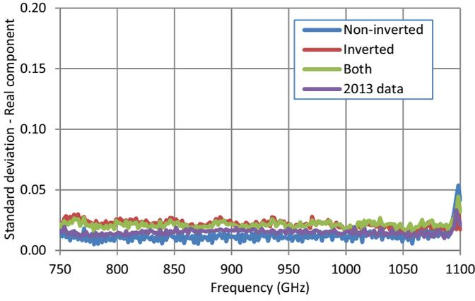
Figure 5:  $s(\Gamma_{R_i}^N)$ ,  $s(\Gamma_{R_i}^I)$  and  $s(\Gamma_{R_i}^{IN})$  for the flush short-circuit. Also shown are the results from 2013
