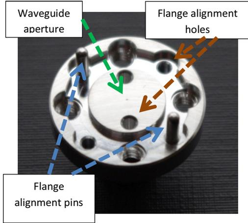
Figure 1: One of the waveguide flanges used during the connection repeatability exercise. The rectangular waveguide aperture is  $250 \mu\text{m} \times 125 \mu\text{m}$  – barely visible to the naked eye
