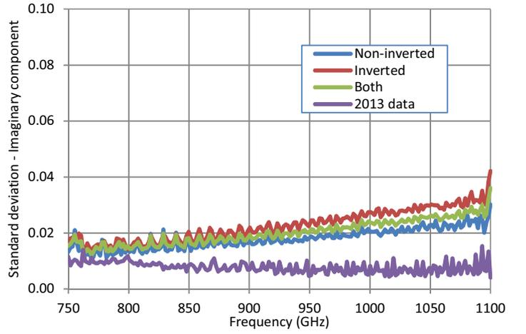
Figure 8:  $s(\Gamma_{I_i}^N)$ ,  $s(\Gamma_{I_i}^I)$  and  $s(\Gamma_{I_i}^{IN})$  for the near-matched load. Also shown are the results from 2013
