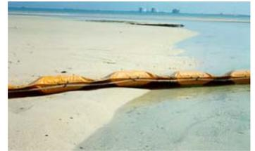
**An oil boom is permanently placed at the creek inlet**
