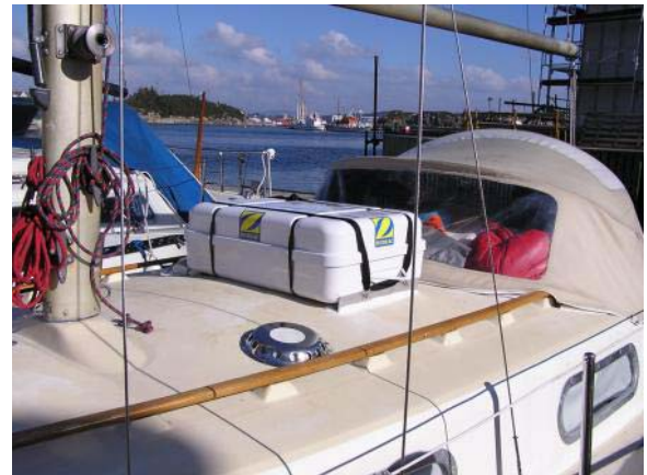
The life raft is strapped to two aluminium profiles, fixed through the deck with six bolts.
