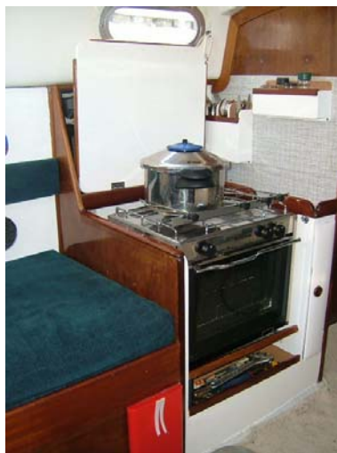
The smallest Techimpex oven fitted nicely. Henrik made a sunken shelf behind it, a heavy tools locker under it, and a plate to use as an extra table when not cooking. The VHF is placed behind the oven, as well as a locker with plastic sliding doors, for sweets and treats.
