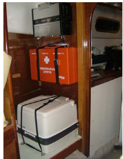
We removed the head and replaced it with the smallest Portapotti. The Wallas heater is convenient in cold weather, and we also found space for the first aid kit.
