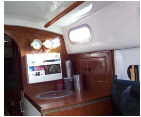
We made an insulated icebox where the sink once were. We cool it with frozen water cans, and drink the water afterwards. In the tropics it'll be an insect-proof locker.
