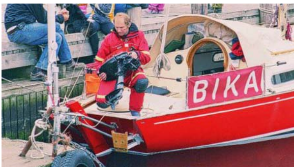
Our handyman, Håkon Evjent, also helped us make an outboard bracket. The 4HP outboard stores on the old inboard engine sole when not in use.
