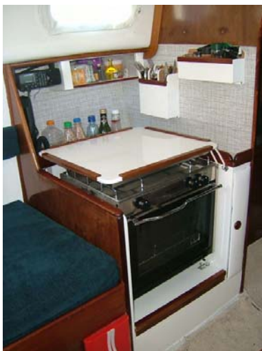
The smallest Techimpex oven fitted nicely. Henrik made a sunken shelf behind it, a heavy tools locker under it, and a plate to use as an extra table when not cooking. The VHF is placed behind the oven, as well as a locker with plastic sliding doors, for sweets and treats.
