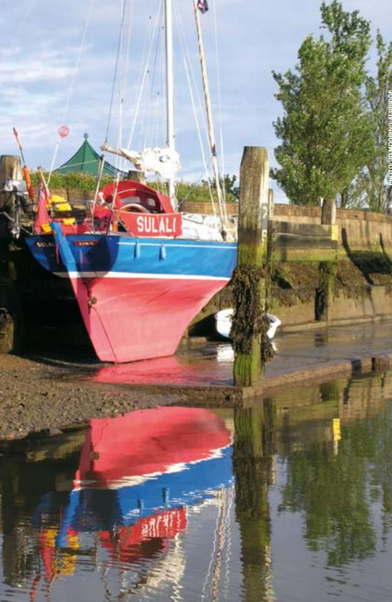
Left Jo Mooring-Aldridge's Sulali dries out, showing the Contessa's deep and long keel with its horizontal base, which many believe is a marked improvement on the Folkboat. Top Jeremy Rogers built his first Folkboat in a garage beside his house in Lymington. Extracting it was tricky. Above The first Contessa 26 hull emerges from Rogers' first Lymington factory.
