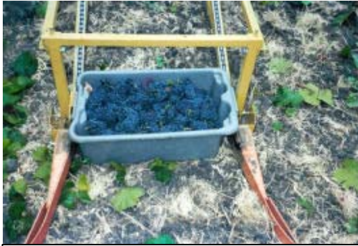
Figure 13: Container pick-up with centering guides.
