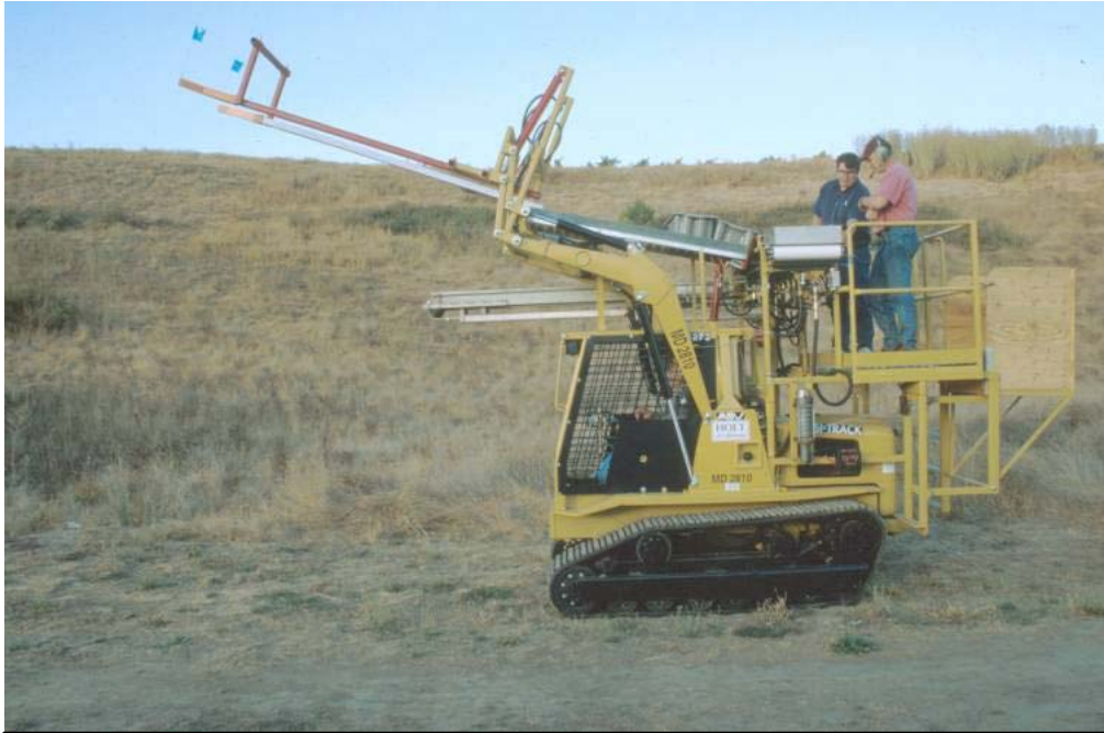
Figure 9: Machine for handling picking containers. Staffing requirements included tractor driver, container handler, and leaf remover.
