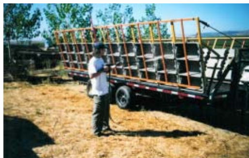
Figure 12: Portable trailer-based container wash rack.
